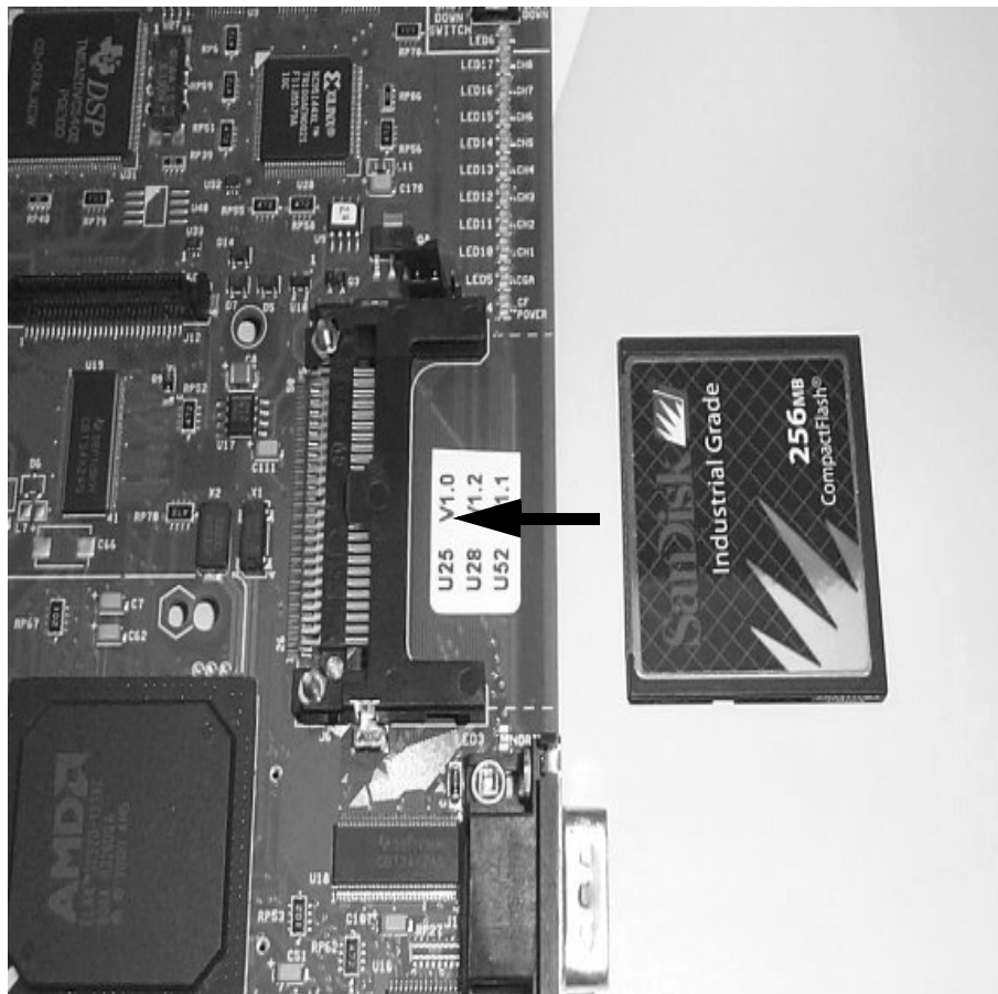
Figure 1 Installing the Flash Drive on the VMP( )-U30 ETU
